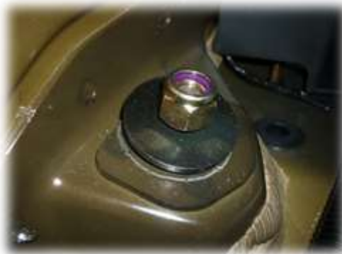
Figure 7: Upper Shock Mount Installation.
