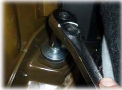
Figure 4: Removal of Factory Shock Absorbers.
