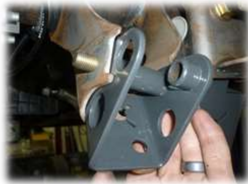
Figure 8: Installing Lower Shock Mounts.
