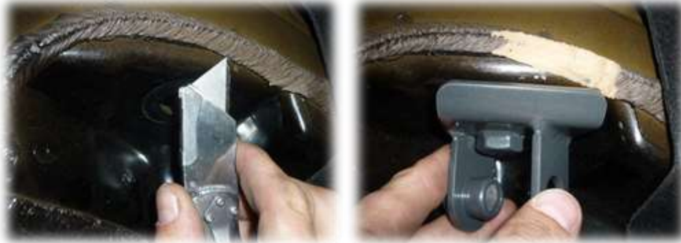
Figure 6: Fitment of Upper Shock Mounts.
