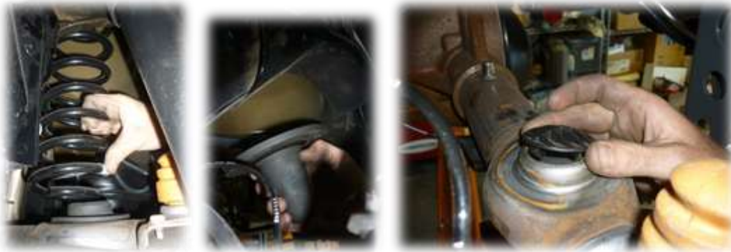
Figure 2: Removing Factory Coil Spring Components.
