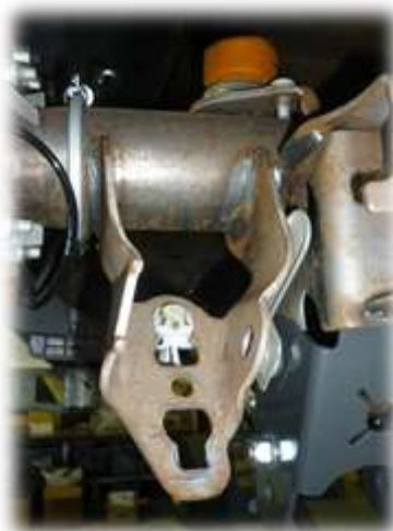
Figure 3: Lower ARB Bolt Removed for Shock Bracket Installation.
