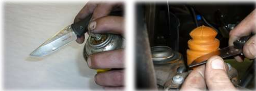
Figure 5: Shortening Factory Bump Stops for Increased Travel.
