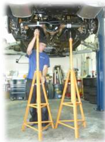
Figure 1: Supporting the Rear End Housing.
