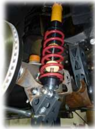
Figure 9: Installed Coil Over.
