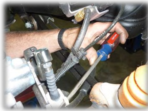
Figure 2: Disconnect Rear Emergency Brake Cables.
