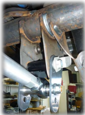
Figure 7: LCA Bracket Installed.
