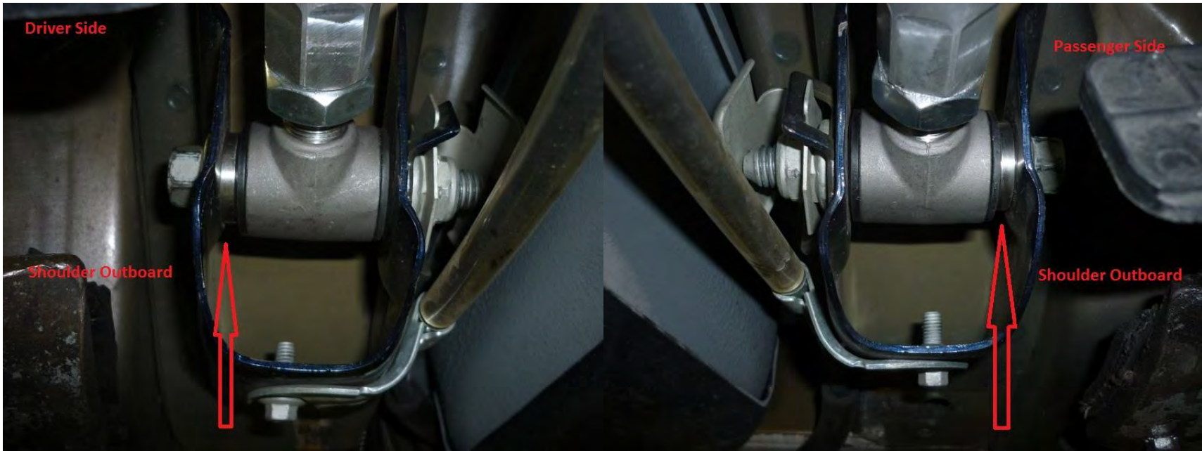
Figure 13: Rear Lower Control Arm Poly Bushing Installations.
