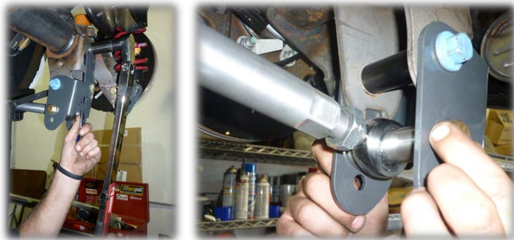
Figure 9: Passenger Side LCA Bracket Installation.
