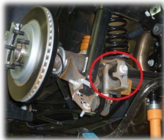
Figure 5: Panhard Bar Bolt Removal.
