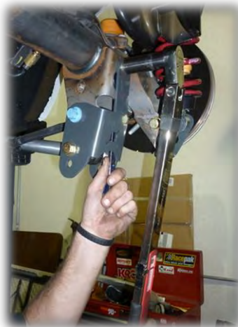
Figure 11: Final Torque of all Fasteners.
