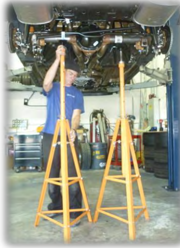
Figure 1: Supporting the Rear End Housing.
