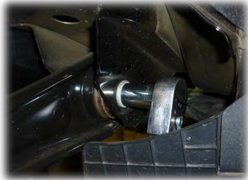
Figure 4: Rear Lower Control Arm Removal.
