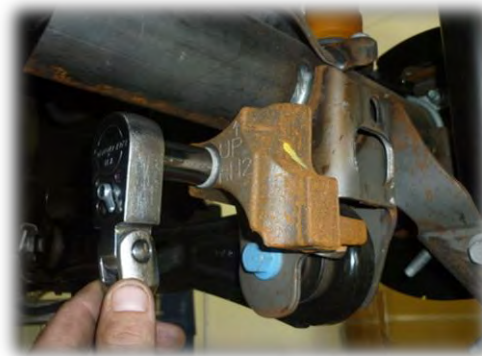
Figure 3: Axle Weight Removal.
