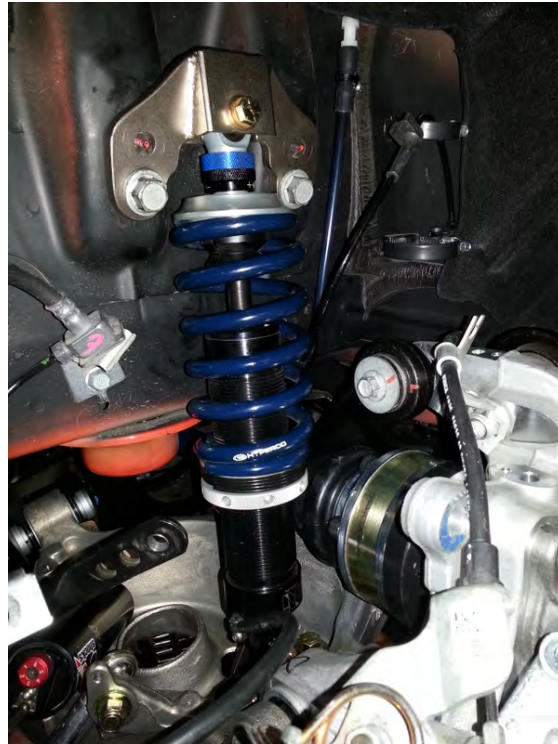
Figure 9: Installed Coil Over. Add correct pictures. This one is out of date.
