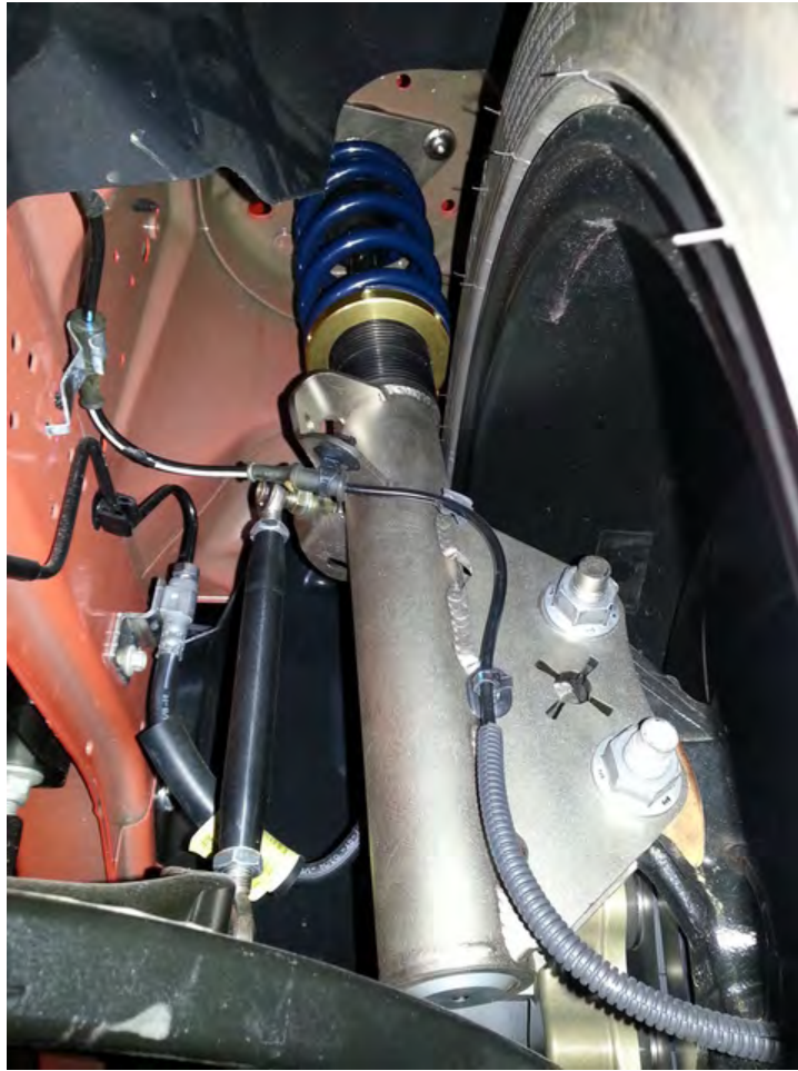
Figure 12: Front Strut Assembly Installed.
